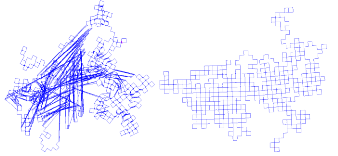
Fig. 5. Minimization of a graph of constraints between poses, before (left), and after (right) the minimization, computed with a GTX280 in 0,65 secs.
