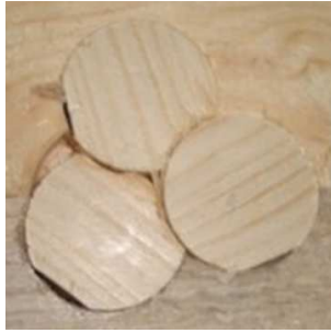
Fig. 2 Defect covered with three patches.
