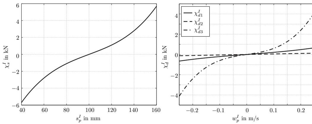
Figure 3. Desired nonlinear stiffness characteristics  $\chi_s^I(s_p^I)$  and damping characteristics  $\chi_{di}^I(w_p^I)$  according to (31) and (32) with parameters given in Table II.
