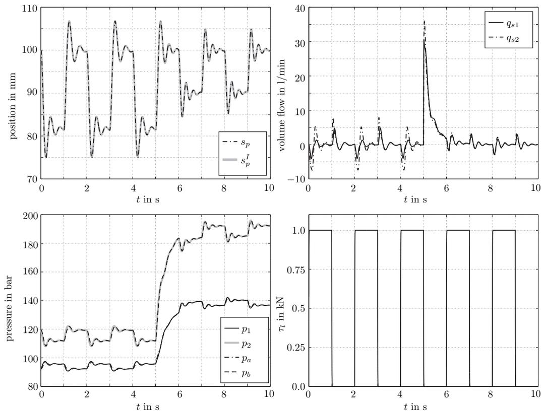
Figure 9. Change of  $\sigma_1$  from  $\sigma_1 = c_1^I$  to  $\sigma_1 = 2c_1^I$  at time  $t = 5$  s for the extended electrohydraulic system.
