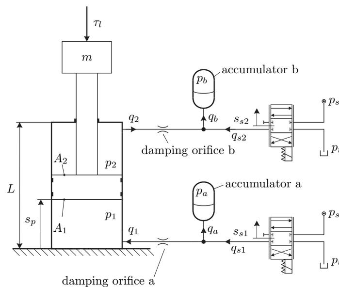
Figure 7. Extended electrohydraulic impedance system.
