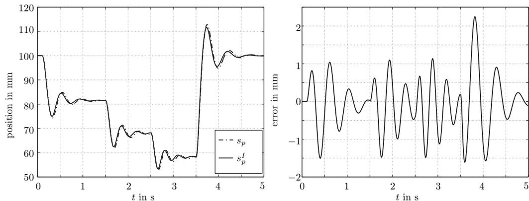
Figure 6. Simulation result of the electrohydraulic system  $\Sigma$  with the I&I based controller (29) and an industrial valve with parameters given in Table I.
