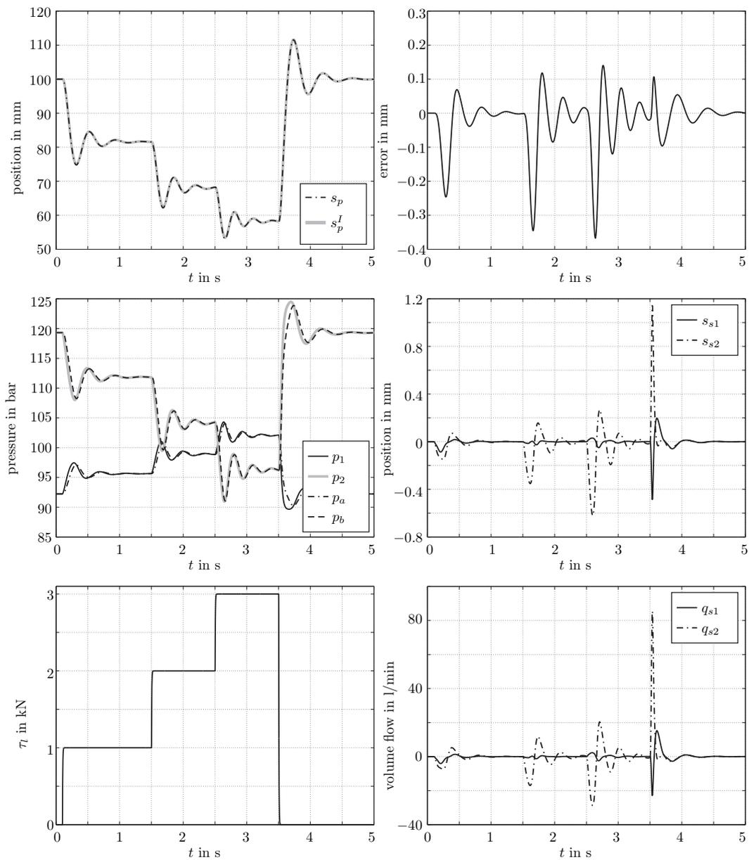
Figure 8. Simulation results of the extended electrohydraulic system in combination with the I&I based impedance control strategy.
