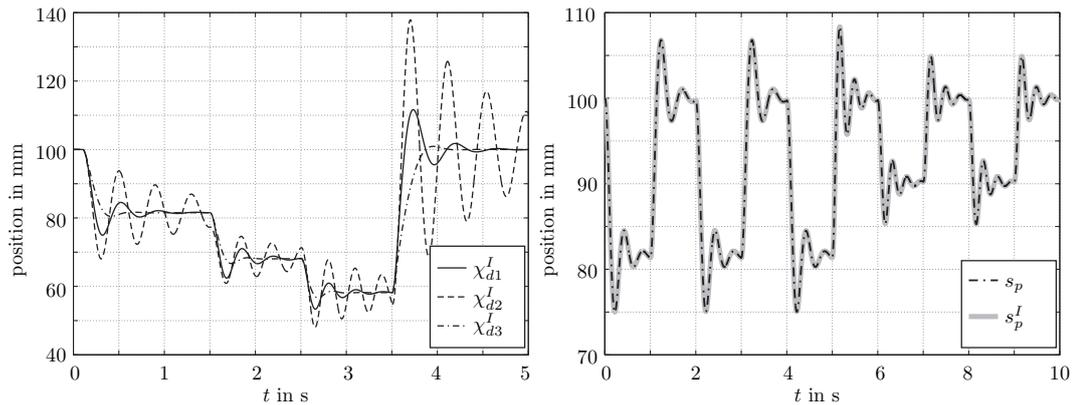
Figure 5. Change of the desired damping characteristics  $\chi_d^I$  and of the desired spring characteristics  $\chi_s^I$ .
