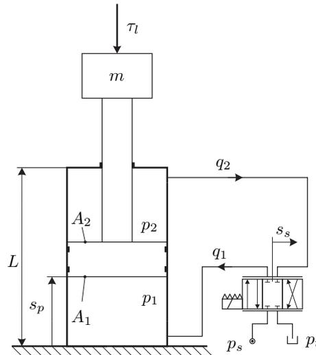
Figure 1. Basic electrohydraulic system used in the impedance control task.
