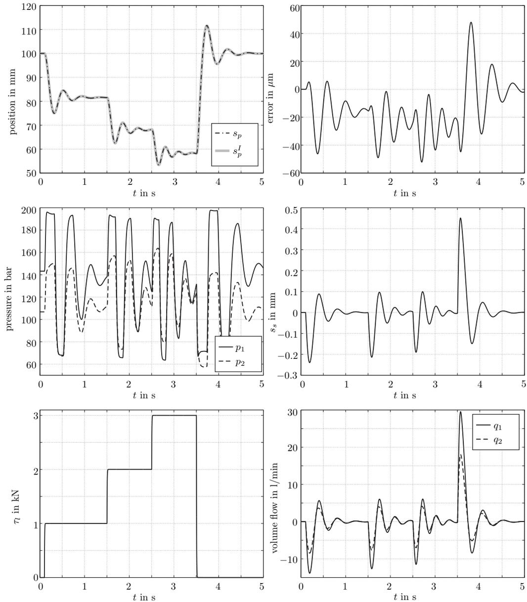
Figure 4. Simulation results for the nominal electrohydraulic system  $\Sigma$  with the I&I based controller (29), the desired spring characteristics  $\chi_s^I$  (31) and the desired damping characteristics  $\chi_{d1}^I$  (32) with parameters given in Table II.
