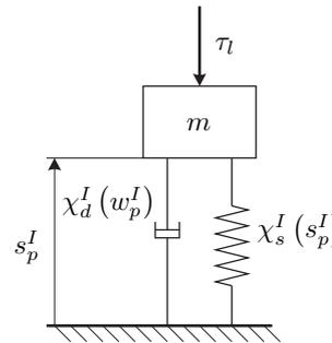
Figure 2. Desired mechanical impedance system  $\Sigma^I$ .
