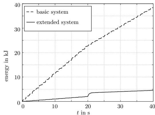
Figure 10. Comparison of the consumed energy of the basic (cf. Fig. 1) and the extended electrohydraulic impedance system (cf. Fig. 7).
