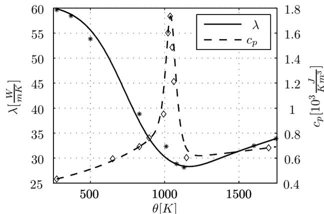
Figure 3. Tabulated values marked with \* and  $\diamond$  and approximating functions of  $\lambda(\theta)$  and  $\rho c_p(\theta)$ , respectively.
