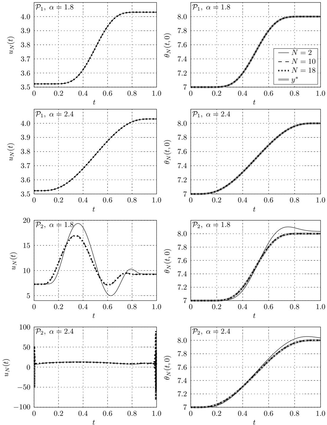
Figure 1. Control input  $u_N(t)$  and output trajectories  $\theta_N(t,0)$  for the trajectory planning of the DCR-system for the parameter sets  $\mathcal{P}_1$  and  $\mathcal{P}_2$ , desired trajectories of different Gevrey classes  $\alpha$  and different numbers  $N$  of grid elements.
