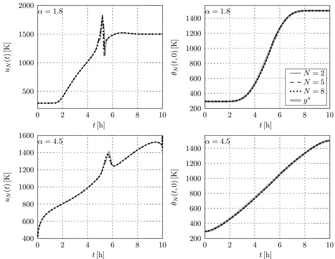
Figure 4. Control inputs  $u_N(t)$  and output trajectories  $\theta_N(t,0)$  for the trajectory planning of the heat-up process for desired output trajectories of different Gevrey classes  $\alpha$  and different numbers  $N$  of grid elements.
