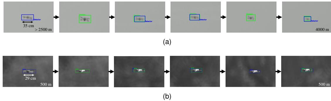
Fig. 8. Two example UAV tracks captured with the proposed telescope system showing a track of the DJI Mavic 3 in front of a clear background in distances between 2500 m and 4000 m. (a) and the DJI Mini 2 in front of a complex background in a distance of 500 m (b). The blue and green boxes visualize the detector and tracker bounding box respectively.
