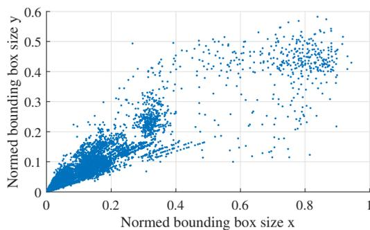
Fig. 3. Each point represents the size of a bounding box, showing the distribution of the bounding box sizes within the training dataset. The bounding boxes are normalized to the image width and height.
