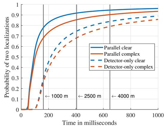
Fig. 7. The probability of two correct UAV localizations, which are necessary for a flight path estimation, within a given time span. The parallel architecture using the reliability-based strategy is compared to a non-parallel detector-only approach. The vertical lines show the minimum duration a DJI Mavic 3 remains within the FoV of the system at different distances.
