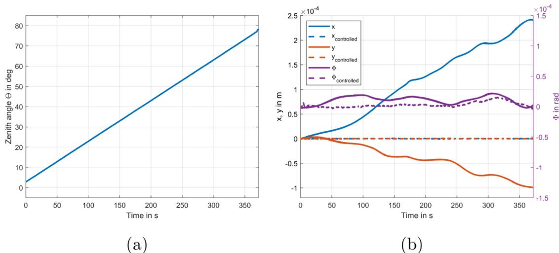
Figure 8: (a) Zenith angle obtained by the absolute encoder over time during slewing. (b) Displacements of the mirror in 3 DOFs without (solid lines) and with (dashed lines) control.<sup>19</sup>
