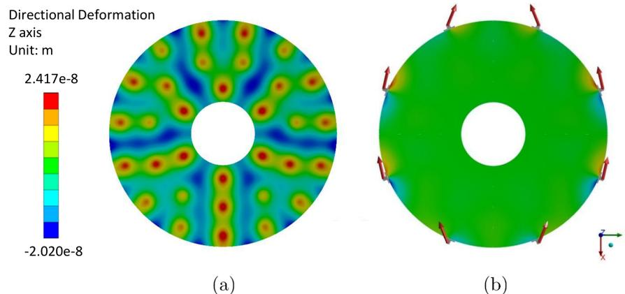
Figure 2: Design results for the primary mirror active optics system. (a) Axial system with 32 supports in three rings. The RMS and PV surface errors are 8.7 nm and 42.4 nm, respectively. (b) Lateral support system with 8 actuators and  $\beta = 0.704$ . The RMS and PV errors when pointing to horizon are 2.3 nm and 40.5 nm, respectively.
