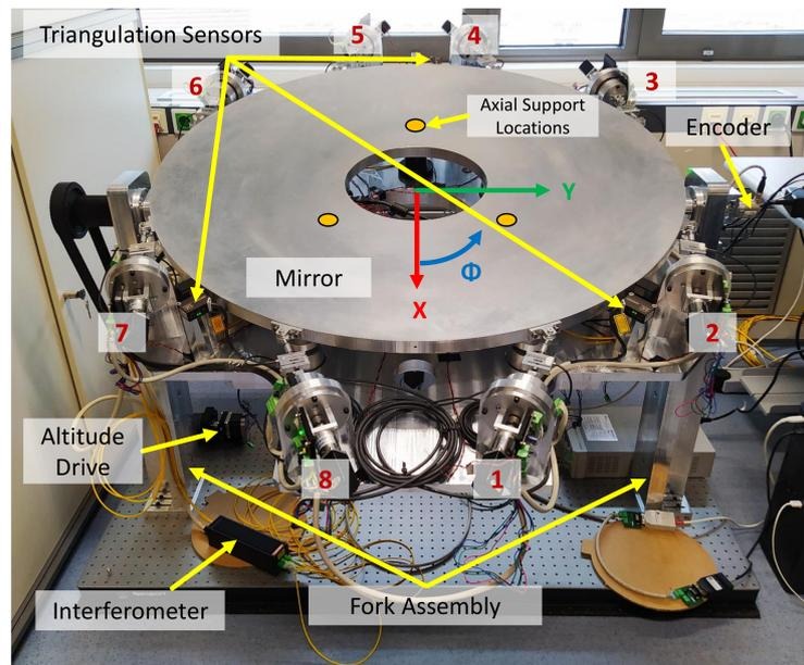
Figure 5: Laboratory setup with aluminum mirror, slewable in elevation axis. Three laser triangulation sensors determine the mirror's position with respect to its cell in 3 DOFs. The 8 lateral actuators are placed at the mirror's circumference.
