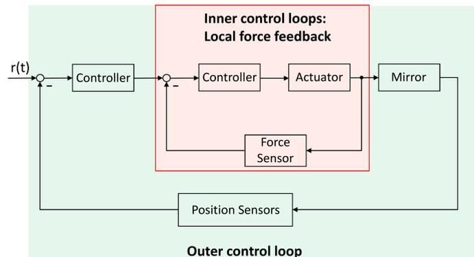
Figure 7: Cascaded control loop with local force feedback on every lateral actuator and position feedback in the outer loop.
