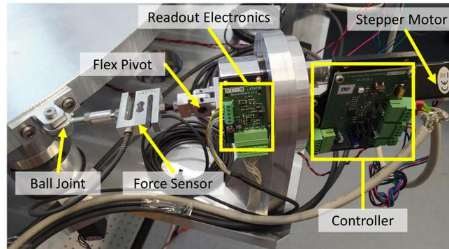
Figure 6: Lateral actuator with ball joint, flex pivot and commercial strain gauge force sensor.
