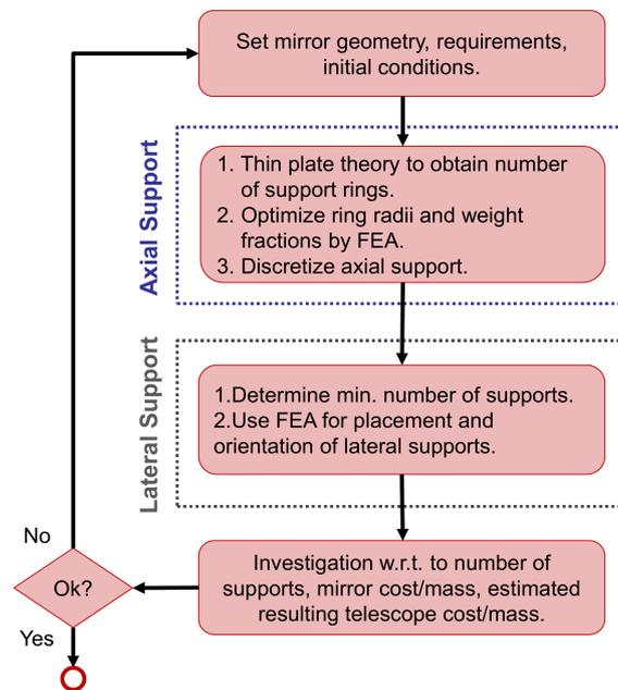
Figure 1: Flowchart of the proposed methodology for designing an active optics support.
