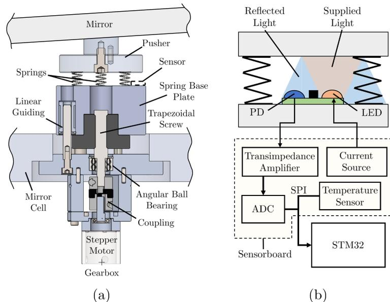
Figure 3: (a) Cross-section view of the electromechanical axial actuator with spring arrangement to achieve desired range and resolution. (b) Optical force sensor based on LED and PD on a compact PCB for seamless integration into the actuator.
