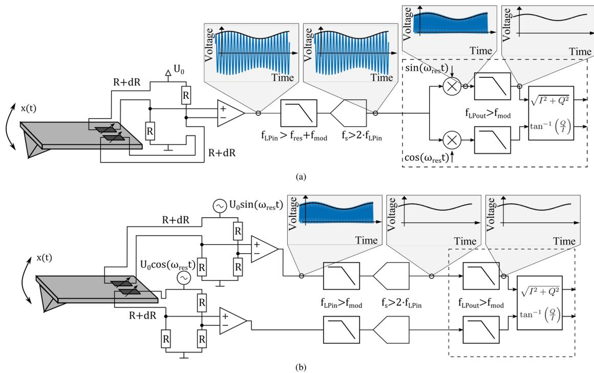
Fig. 1: Illustration of piezoresistive deflection measurement and demodulation of AFM cantilever oscillation. (a) Conventional demodulation by lock-in amplifier. (b) Mechatronic demodulation.
