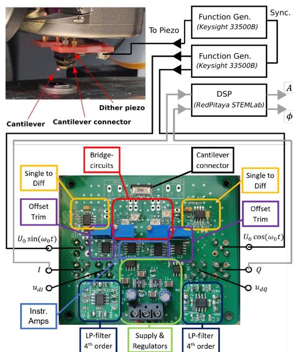
Fig. 2: Close-up of the cantilever holder, image of the custom-built PCB and block diagram of the demodulation method. The figure is adapted from [17].
