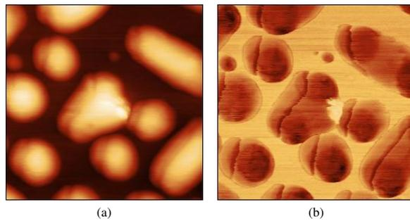
Fig. 5: AM-AFM images of PS-LDPE sample using mechatronic demodulation. The scan size is  $10 \times 10 \mu\text{m}$  and the scan rate is 0.25 lines/second. (a) Topography image (range of color scale is 200 nm). (b) Phase image (range of color scale is  $6^\circ$ ).
