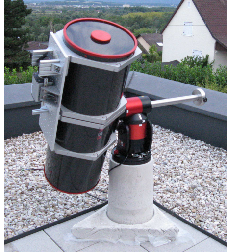
Figure 1: Investigated satellite tracking system developed together with ASA Astrosysteme GmbH, mounted on a test site in Upper Austria. Also visible on top of the tube is the optical breadboard with tertiary mirror and camera.
