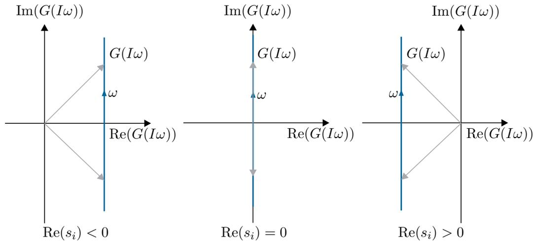
Abbildung 4.16: Stetige Winkeländerung von  $(s - s_i)$ .
