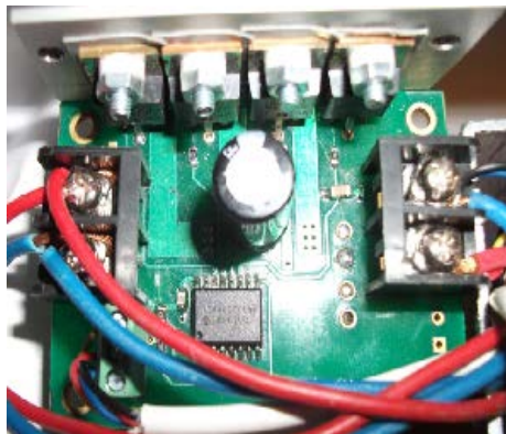
Fig.10. H-Bridge used in the system
