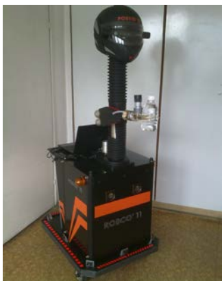
Fig.1 ROBCO 11 - Intelligent Modular Service Mobile Robot for Elderly Care
