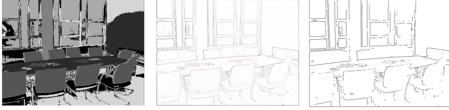
Figure 1.4: 2D scene geometry: the left image shows a region segmentation based on a color clustering; in the middle a Difference of Gaussian (DoG) filter has been applied to the original image; the right image shows a contour segmentation based on the DoG image.
