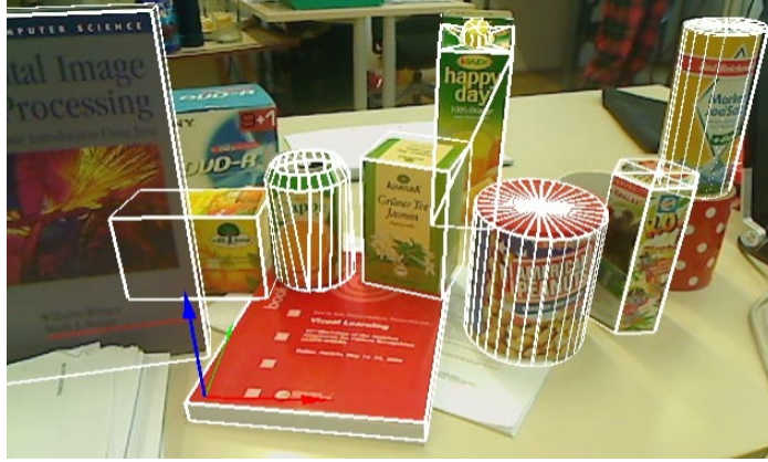
Figure 1.10: An example scene where objects have been recognised based on their main structure (displayed) and are then tracked using the superimposed texture taken from the actual objects [55].
