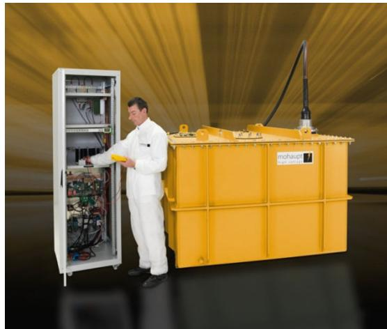
Fig. 1. On Site Test System DRT200-1, 200 kV, 1  $\mu$ F
