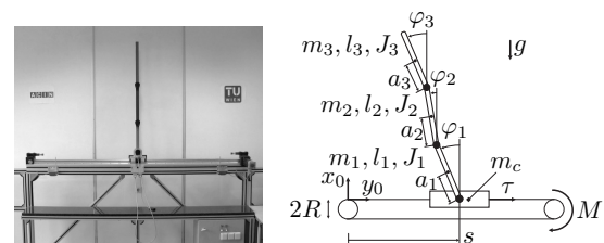
(a) Photograph of the test bench. (b) Schematics of the triple pendulum on a cart.
